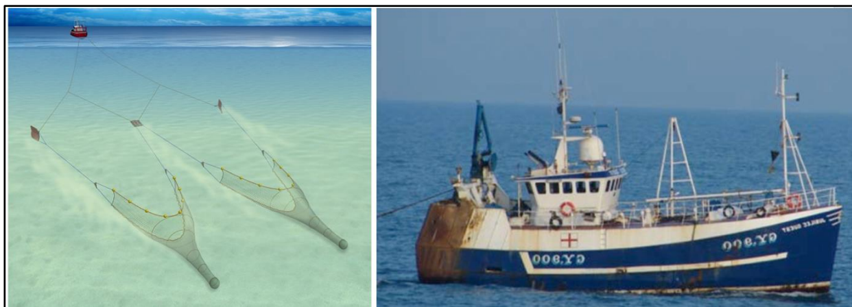
Figure 28: Typical demersal otter trawler vessel and gear diagram (Sources: Visserijnieuws, 2010; Seafish, 2019).
